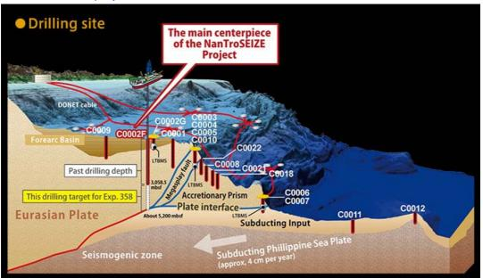
Yan: Oceanic plate comes from here, is subducting under Japan Island, convecting sediment of ocean floor forms "Accretionary prism".
