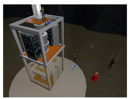
Yan: If Drill Pipe penetrates oil or gas reserver, usually pressure inside of drill hole is controlled, but once fails well control, oil or gas like Hydrocarbon or Hydrogen Sulfide ascend through Riser pipes and is released on the Moon Pool area and Drill Floor directory. Then, this BOP cuts off the drill pipe and shuts off the well.
