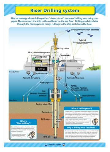
Yan: This is "Drill Pipe". Total 9 km length. At first, sea water is sending through Drill Pipes to discharge cuttings out from hole.
