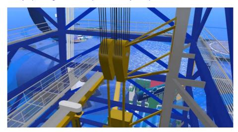
Yan: This is "Top Drive" or "Power Swivel" rotates drill pipes and above of Top Drive is "Travelling Block" which can hang 900 tons.
